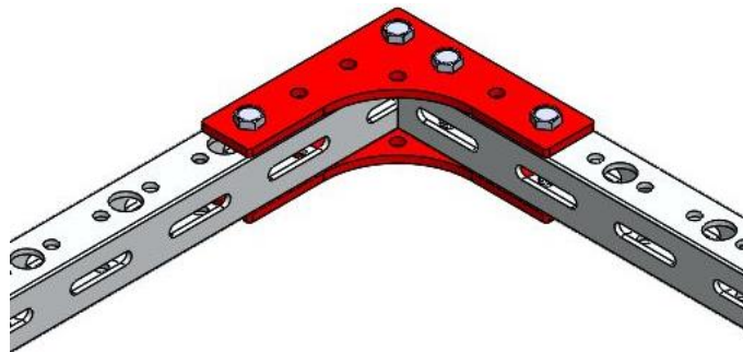
Figure 13: Gussets on both sides of the joint
